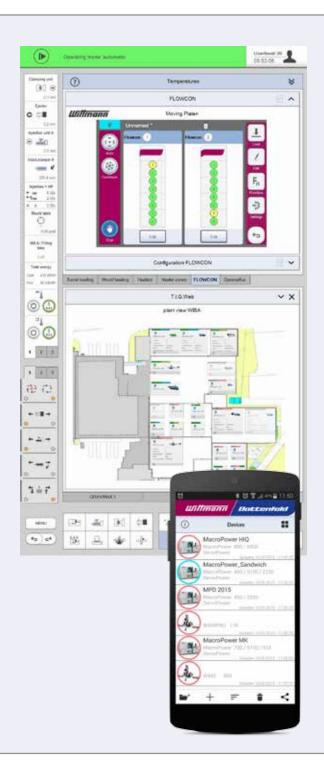
With its internal communication standard WITTMANN 4.0, the WITTMANN group offers a uniform, data transfer platform between injection molding machines and peripheral equipment from WITTMANN. For an appliance exchange, the correct operating software is loaded automatically via an update function according to the "plug & produce" principle.
