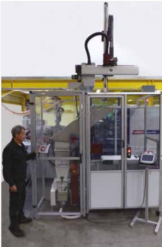
G-Max 12 – inside workcell placed under a chute
