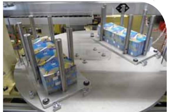
Vertical magazine for large labels
