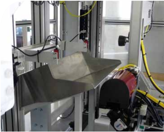
Label detection: color sensor
