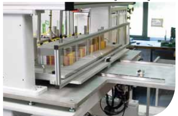
Vertical magazine for large labels
