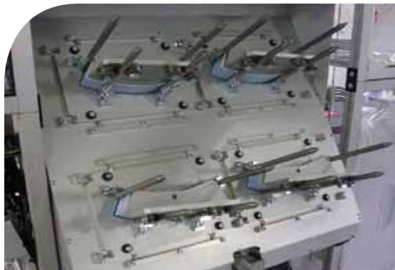
Cost efficient horizontal magazine for flat labels
