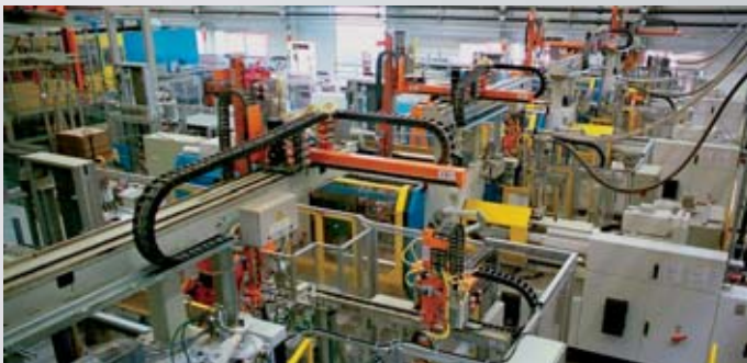
A car maker's fully automatic plant: four 4,200 kN machines producing hybrid bars as metal-plastic composites. Demag linear robots place the metal inserts in the moving half of the mould and remove the finished parts from the fixed half.
