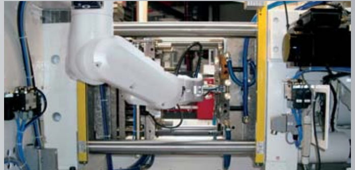
Production cell for medical devices: a 6-axes robot is suspended in the cleanroom housing from a cantilever at the side of the Demag machine. This compact layout offers small masses to be moved and ensures short paths from the point of part removal to the stacking station.
