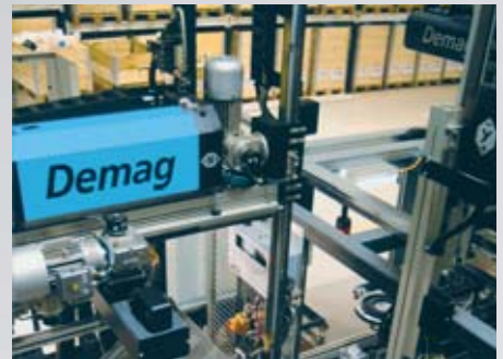
Integrated into a production cell with multiple assembly, decoration and inspection functions – shown here in a moulding shop producing stackable plastic containers – the Demag robot separates sprues and feeds the moulded parts one at a time to the downstream finishing stations.
