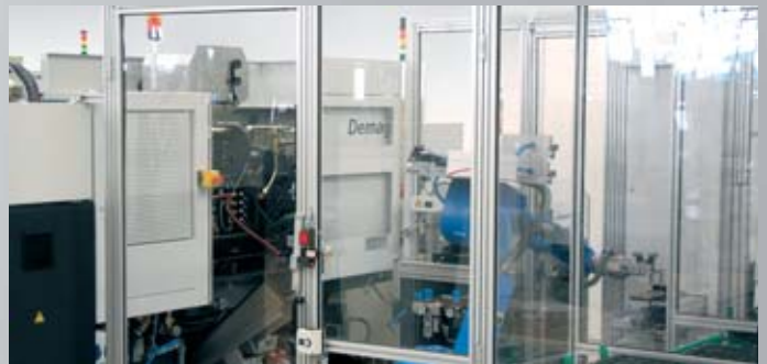
Fully automatic production cell operated by a manufacturer of mobile phone displays: 6-axes robots remove the IMD mouldings from the Demag IM machine, delivering them to cleaning stations, inspection systems (in background) and workpiece carriers (in foreground).
